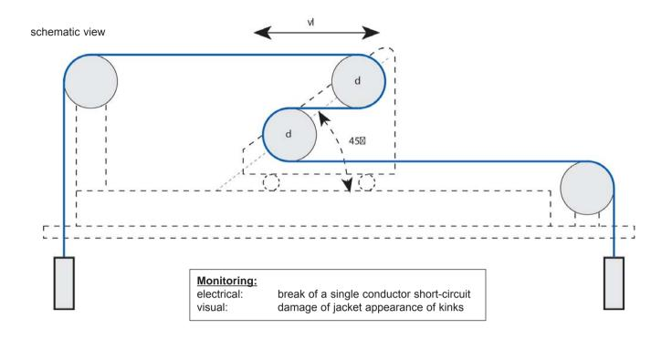
Test construction acc. to DIN VDE 0281 part 2 (HD 21.2 S3), for PVC insulated cables.
