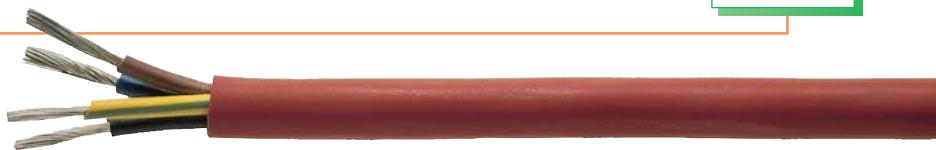
BiHF-J is a multi-conductor, silicone insulated control cable with a reddish brown silicone jacket. Silicone cables are recommended for use where high temperatures rapidly cause other cables to deteriorate. Recommended applications include foundries, steel mills and glass factories and other high temperature processes.
